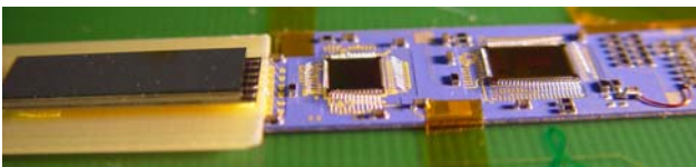
Figure 5: The optical Package, GOL and Digital Pilot positions in the MCM missing optical power margin
