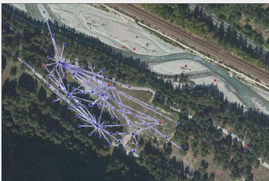
Fig. 1 - Position of the network (red triangle) and detail points (blue circles) used in the geodetic survey of the study area (Beaulard, Piedmont, northern Italy).
