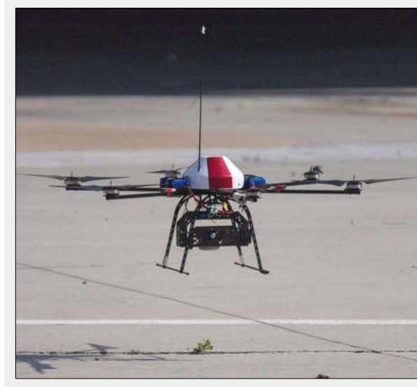
Fig. 2 - UAV used for aerial photogrammetry (Hexakopter®, Mikrokopter, Moormerland, Germany).
