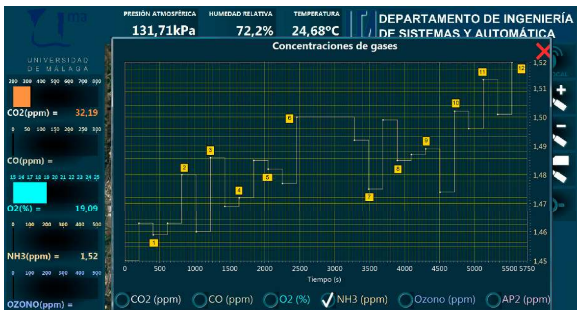
Figure 14. Measurements for the NH3 sensor obtained in a networked mode experiment, as shown by the user interface.
