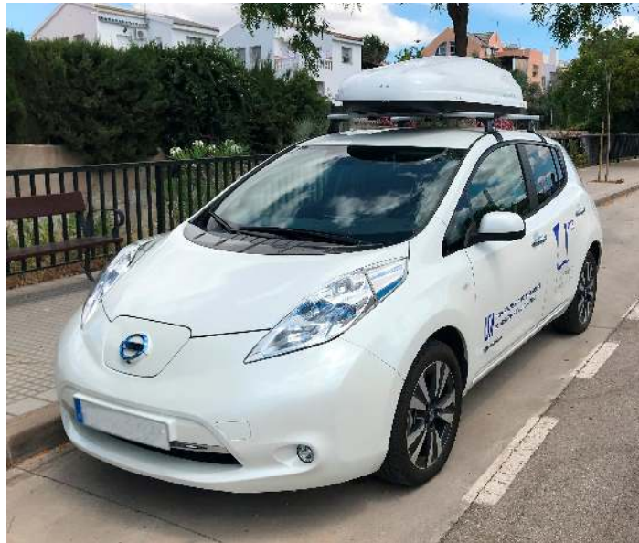
Figure 11. Vehicle used in experiments showing the top case with the UIS Mobile node installed.
