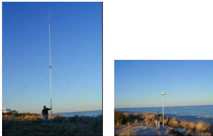
Figure A-1. Transmit (left) and receive (right) antennas for a typical CODAR-type long-range system.
