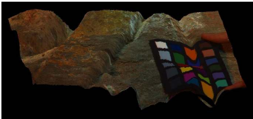
Figure 4: Multispectral data as texture on a 3D model. The mapping is incorrect where the Macbeth chart and fingers are shown because they are not part of the 3D scans.
