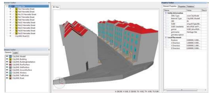
Figure 17. CityGML Model Showing Semantic Classes.
