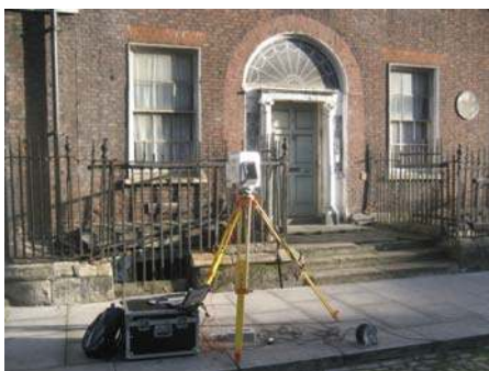
Figure 9. Trimble GS200 Laser Scanner
