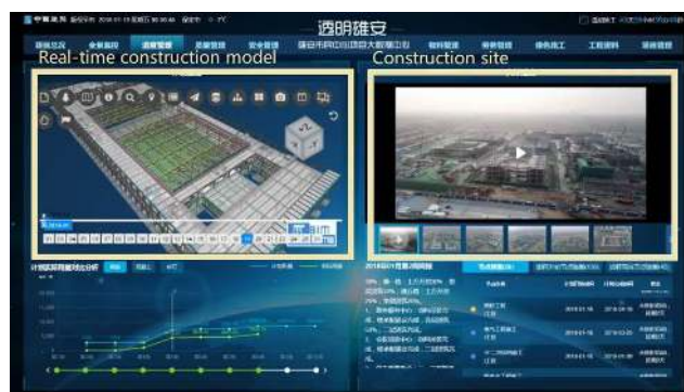
FIGURE 7. Digital twin of the construction in progress.
