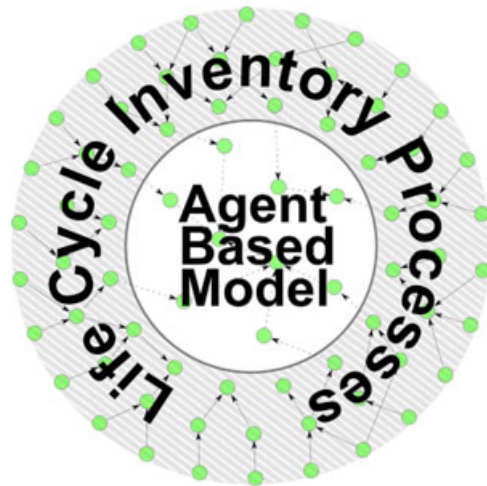
Figure 5 Systems representation in the hybrid model. Dynamic supply chains in the agent-based model connect to static, predefined supply chains.
