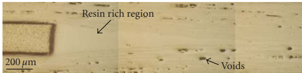
FIGURE 3: Photomicrograph of the resin pocket area around the embedded dummy sensor: side view (along the fiber direction).
