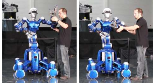
Fig. 5. Initial configuration (left) and snapshot during the experiment #1 (right) on self-collision avoidance. Except for the left arm (7 DOF), all other joints are locked in order to facilitate repeatability of the experiment.
