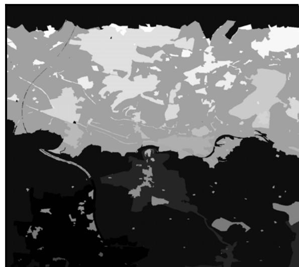
Figure 6: Rasterised and merged extracted vector map polygons. Each agglomerate is given a unique grey value.
