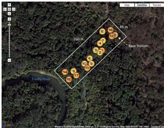
Fig. 9 Sensor deployment topology in the field as shown on the Google Map-based TEO Online web portal
