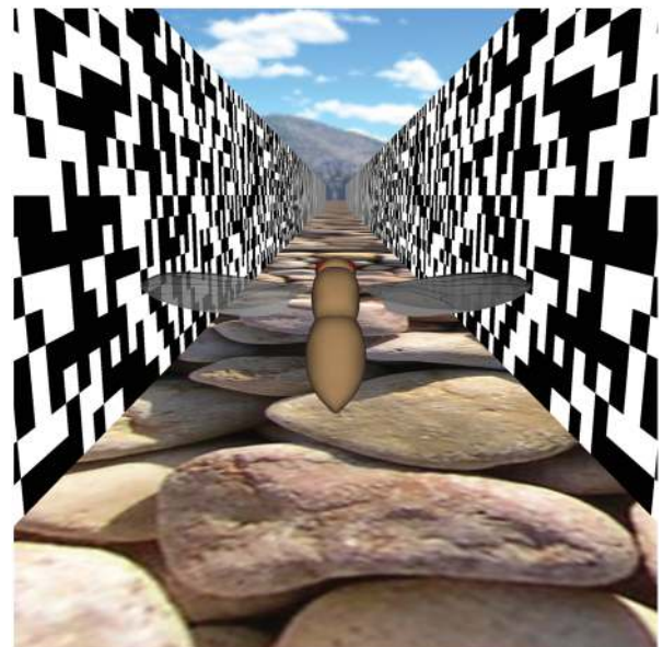
Fig. 8 A view of the simulated 3-D environment within the OpenSceneGraph engine. The position and orientation of the fly's head are used each time step of the simulation to generate images that are optically filtered to provide the visual input to each model photoreceptor.
