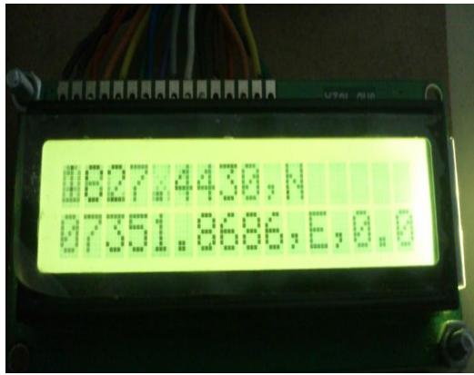
Fig6: vehicle unit and accident location displayed on the LCD
