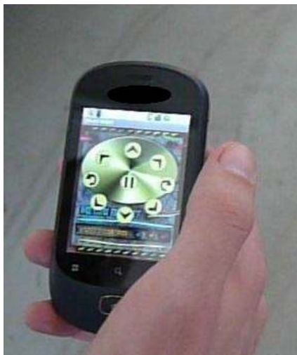
Figure 2. Android mobile phone used as remote control
