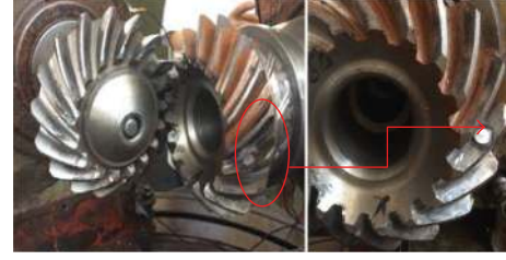
FIGURE 3: Tooth surface pitting.
