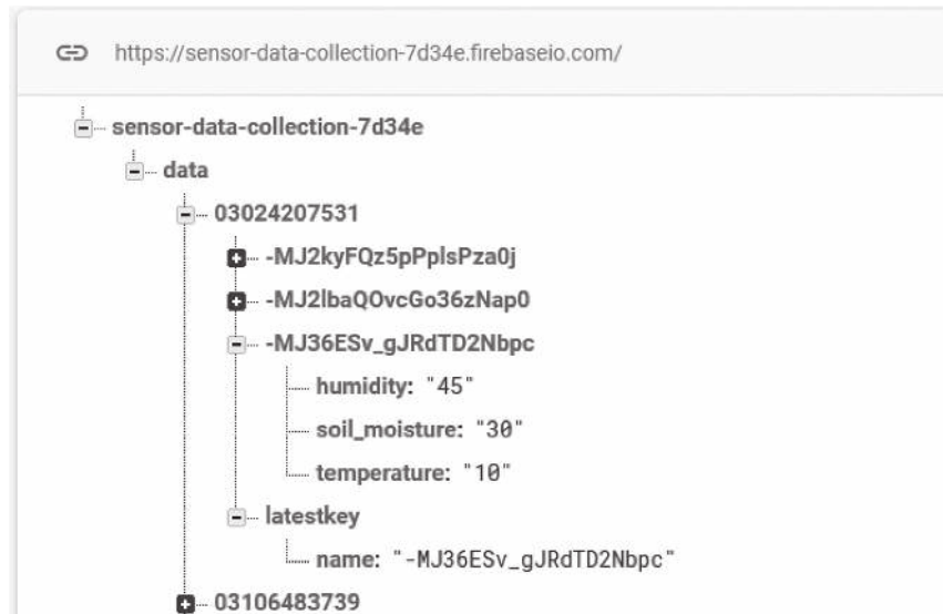
FIGURE 11: Edge server handling data from sensors via the HTTP request.
