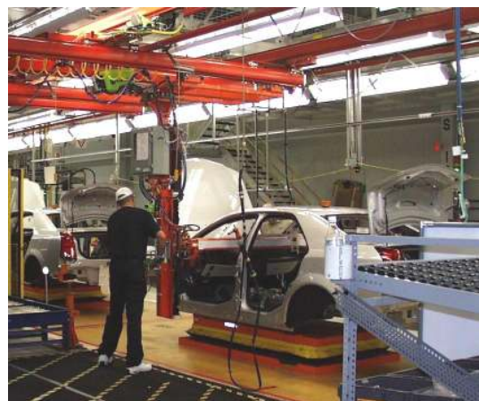
Fig. 4. IAD for cockpit loading. This IAD is capable of semiautonomous motion.
