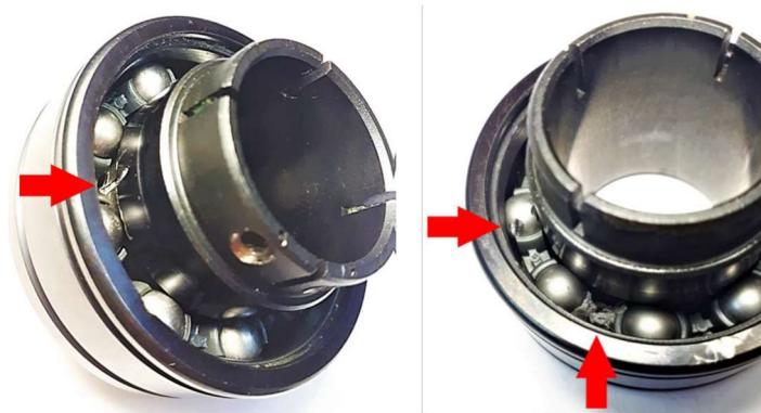
Fig.10. Test-bearings with inner race fault (left) and ball fault (right)
