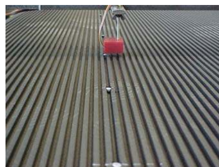
Figure 7.3 Magnets line and sensor
