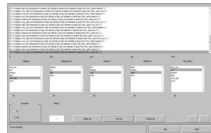
Figure 5. Fuzzy logic rules editor between input & output parameters
