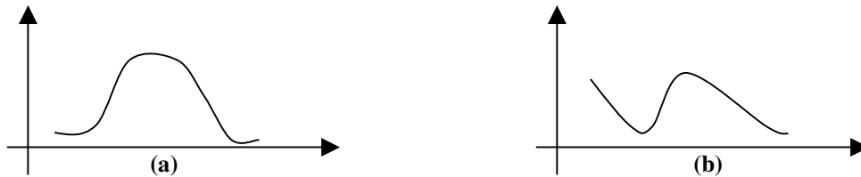
Figure 3. Uni-modal distribution shape on (a) versus a bi-modal distribution shape on (b): the standard deviation of the latter is greater, thus making the latter less significant under the z-scoring standardization, which is odd in the clustering context.
