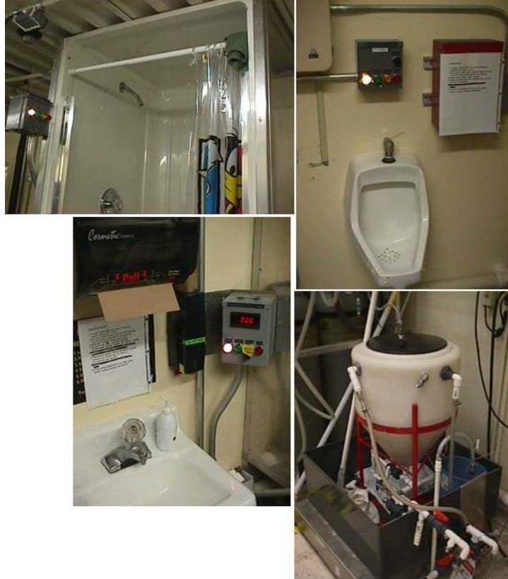
Figure 5 The iWRS waste water collection system. Human volunteers donate urine, showers, and hand washes, using liquid soap with the chemical composition of that to be used on the space station. A computer system responds to the pushbuttons at each donation site to weigh and record each type of donations before sending the donation to the main feed tank for the iWRS. Prepared solutions representing respiration water are added to the feed tank to complete a composition representative of that expected on the space station and/or planetary outposts.
