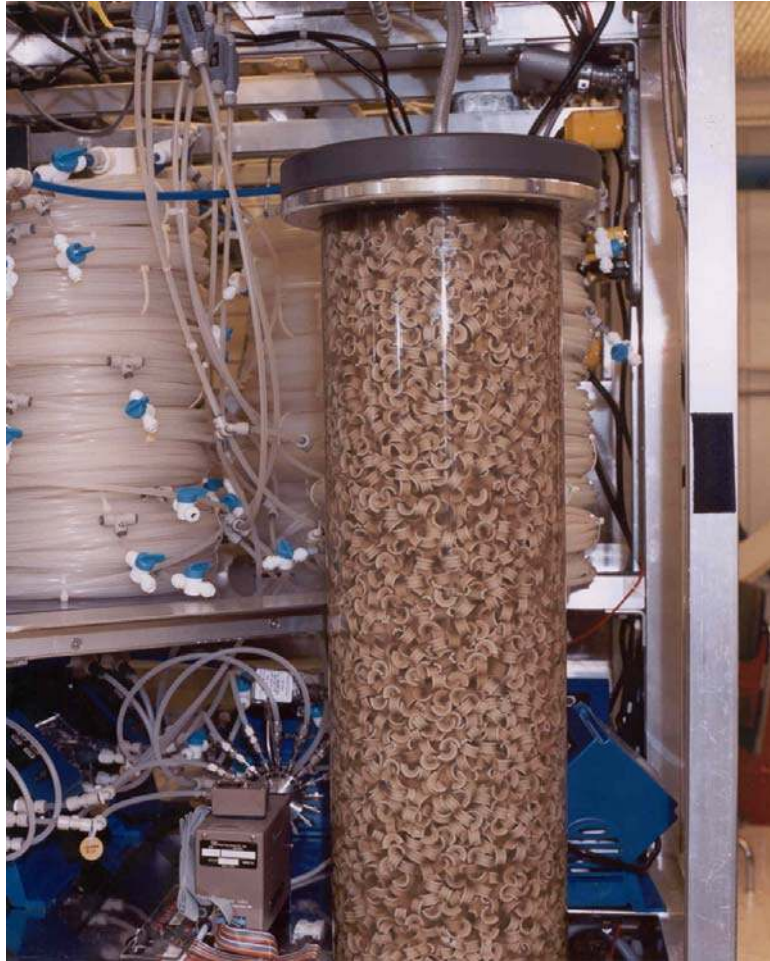
Figure 13 Symbiotic biological reactors. Feed water flows from the packed bed on the right through the nitrifier (eight 300' coils of thin tubes on the left and to the rear), through the GLS (not shown) and back to the packed bed. The nitrifying reactor contains bacteria that use oxygen gas ( O_2 ) to break down the ammonia ( NH_4 ) in the feed water into nitrates ( NO_3 ) and nitrites ( NO_2 ). Bacteria on the ceramic saddles in the packed bed remove organic carbons from the feed water using oxygen from the nitrate and nitrite molecules provided by the nitrifier. The resulting nitrogen and carbon dioxide gases are released in the GLS.
