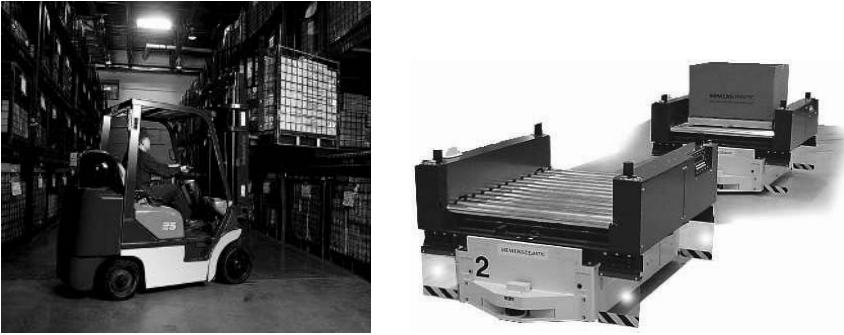
Figure 1.2 A forklift truck in a warehouse (left) and AGVs (right) (courtesy of the Kingdom Group and Siemens Dematic)
