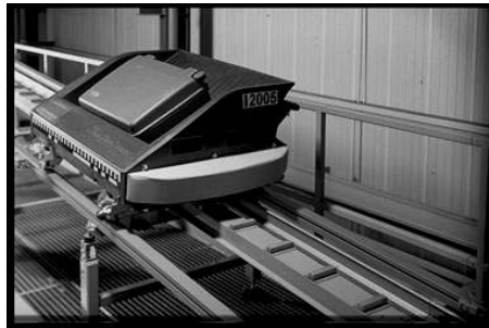
Figure 5.1 A Destination-Coded Vehicle (courtesy of Vanderlande Industries)
