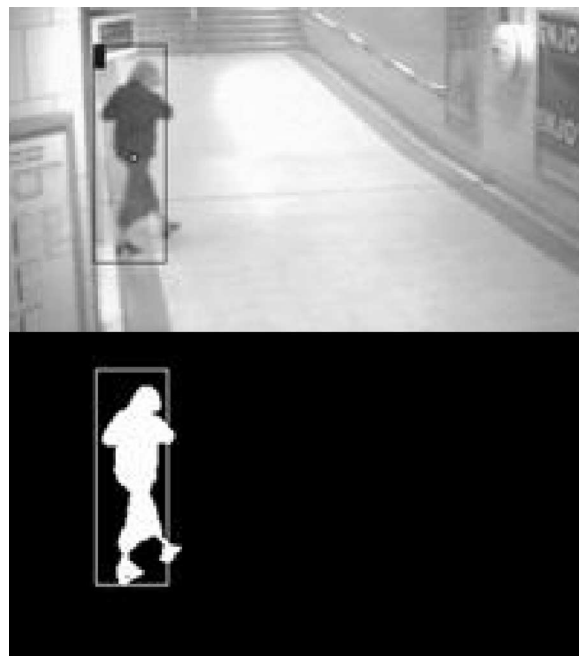
Fig. 3 Example of background subtraction technique used in motion detection. In this example a bounding box is drawn to fit the object detected
