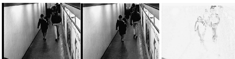
Fig. 2 Example of temporal difference technique used in motion detection
