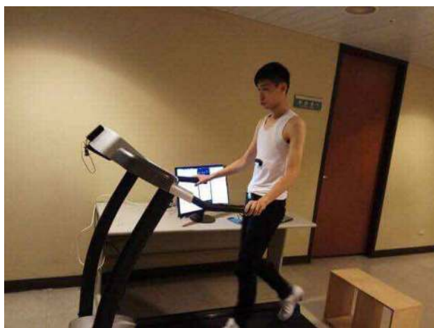
Fig. 2 A subject wearing the smart clothing and exercising under the guidance of the proposed intelligent exercise guidance system. The black object on the white smart clothing is the gateway
