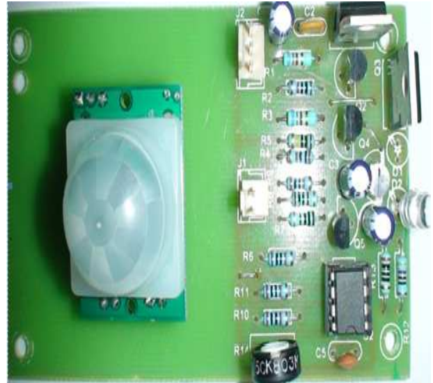
Fig. 11 PCB photo of PIR sensor and IR transmitter
