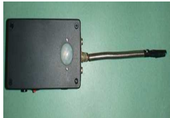
Fig. 12 Casing of IR transmitter
