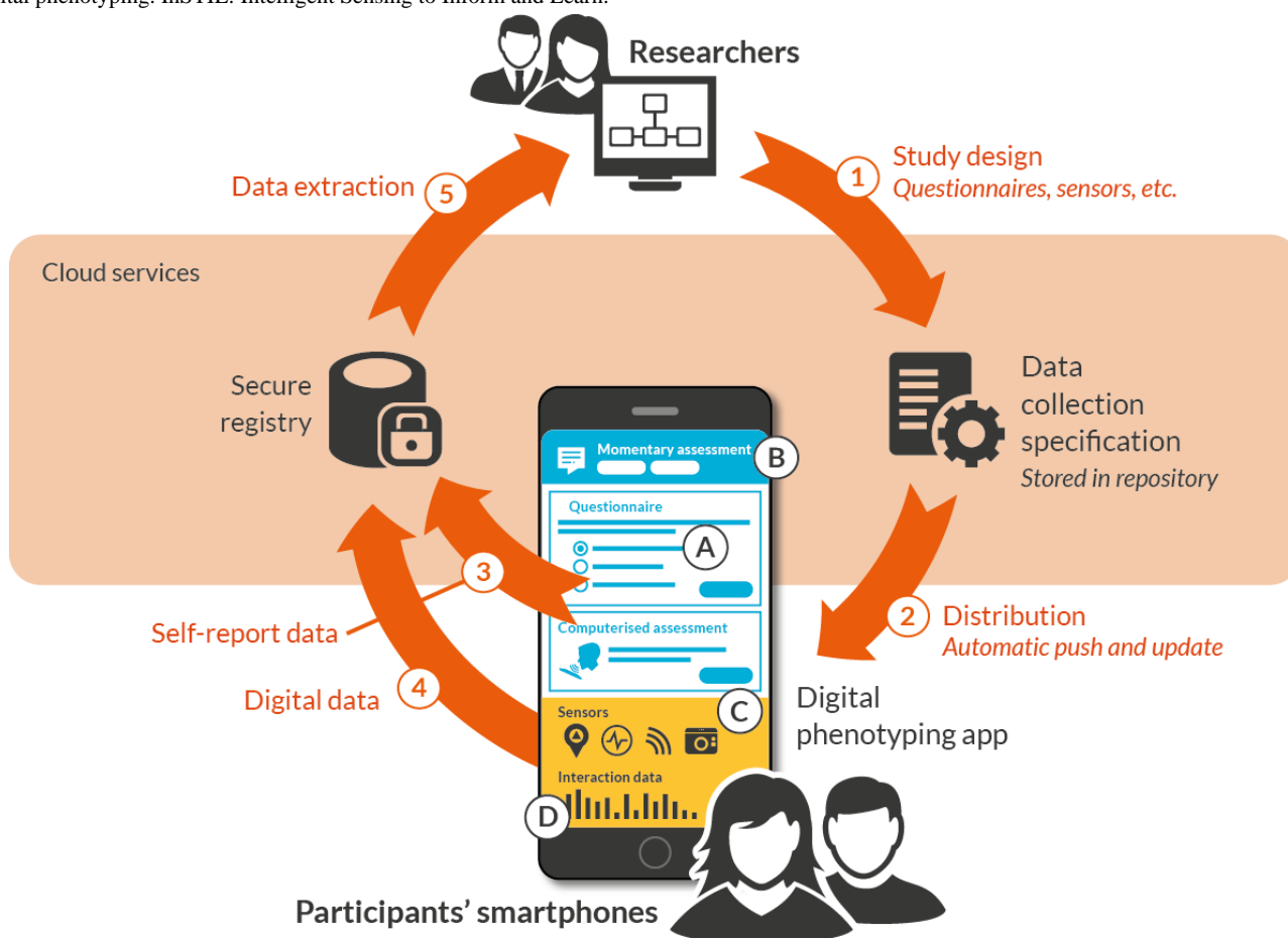
Figure 1. InSTIL Common research workflow. The figure shows how the platform supports a sequence of key activities for researchers involved in digital phenotyping. InSTIL: Intelligent Sensing to Inform and Learn.
