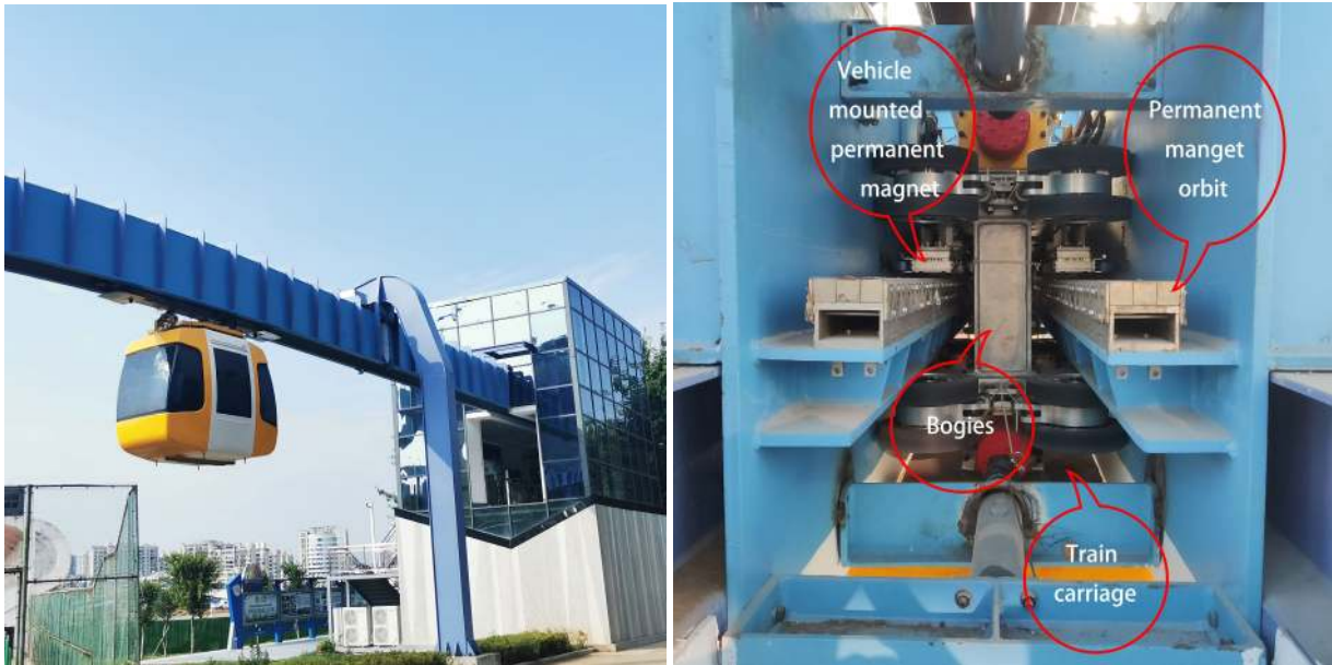
FIGURE 4. Operation and suspension diagram of permanent magnetic maglev train.
