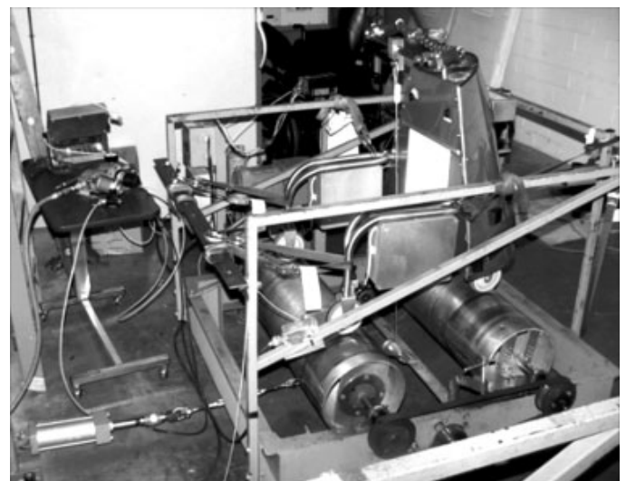
Figure 3. VA-PAMAID on two-drum tester. A cyclic load was applied to handlebars, and the walker completed 200,000 cycles at 1 m/s.
