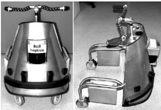
Figure 1. Front and side views of VA-PAMAID walker.
