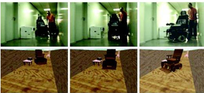
Figure 17. Mixed-reality test: Real intelligent wheelchairs (upper images) interacting with virtual objects (lower images).
