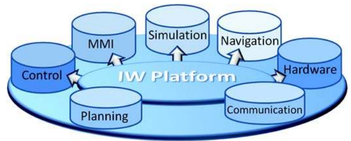
Figure 1. IntellWheels project modules. IW = intelligent wheelchair, MMI = multimodal interface.
