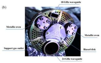
FIG. 3. Conventional components of the SECRAL source: (a) schematic view of the injection tank; (b) photo of the injection tank end.
