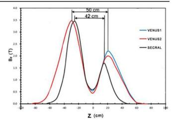
FIG. 21. Comparison of the axial magnetic field distribution between SECRAL and VENUS. (The blue line VENUS1 and the dark line SECRAL are the magnetic field distribution for optimizing high intensity <sup>209</sup>Bi<sup>30+</sup> beam respectively. The red line VENUS2 is the new field distribution for VENUS after modifications.)
