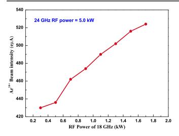
FIG. 20. <sup>40</sup>Ar<sup>14+</sup> beam intensity dependence on microwave power of the second supplemental heating frequency 18 GHz when the main frequency 24 GHz power is fixed.
