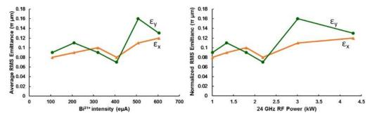
FIG. 24. Dependences of normalized rms emittance on the beam <sup>209</sup>Bi<sup>31+</sup> intensity and the 24 GHz microwave power at SECRAL.
