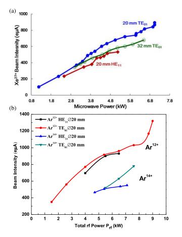
FIG. 17. Dependence of beam intensity on total microwave power at 24 + 18 GHz coupled at different microwave coupling schemes. (a)  $^{129}\text{Xe}^{27+}$  beam; (b)  $^{40}\text{Ar}^{12+}$  and  $^{40}\text{Ar}^{14+}$  beam.
