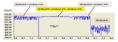
FIG. 26. Suppression effect of beam instabilities by two-frequency heating (28 + 24 GHz) and three-frequency heating (28 + 24 Hz).
