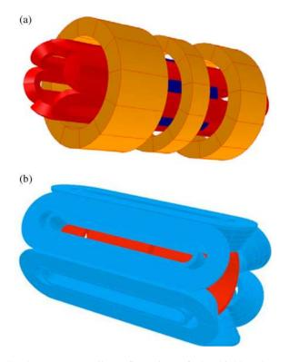
FIG. 5. Magnet coil configuration of the highly charged ECRIS. Classical ECRIS magnet coil configuration of Sext-In-Sol. The SECRAL superconducting magnet coil configuration of Sol-In-Sext.
