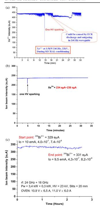
FIG. 27. SECRAL beam stability study. (a) Beam intensity instability of  $^{129}\mathrm{Xe^{27+}}$  at 435 e $\mu\mathrm{A}$  when SECRAL was tested with single frequency 24 GHz heating at 3.5 kW power. (b)  $^{129}\mathrm{Xe^{30+}}$  beam intensity stability at 235 e $\mu\mathrm{A}$  with 24 + 18 GHz. (c)  $^{209}\mathrm{Bi^{31+}}$  beam intensity stability at 330 e $\mu\mathrm{A}$  testing continuously during 2.5 hours.
