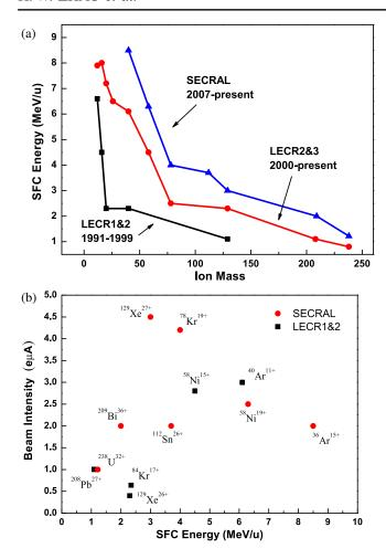
FIG. 29. Enhancement of SFC cyclotron beam energy and beam intensity due to SECRAL operation. (a) SFC beam energy improvement by SECRAL compared with the normal conducting ECR ion sources LECR0&1 and LECR2&3. (b) Enhancement of SFC beam intensity and energy by SECRAL compared with the normal conducting ECR ion sources LECR2&3.
