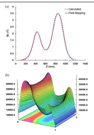
FIG. 9. SECRAL axial magnetic field distribution. (a) Designed axial mirror magnetic field ( $B_z$ ) distribution on the axis for SECRAL 24–28 GHz operation. (b) 3D field distribution at the x-z plane in the plasma chamber.
