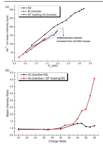
FIG. 13. Xenon beam intensity study with different chamber and microwave power. (a)  $^{129}\mathrm{Xe^{27+}}$  beam intensity evolution as a function of microwave power and comparison among stainless steel (SS) chamber at 18 GHz, aluminum (Al) chamber at 18 GHz, and aluminum chamber at 18 + 14.5 GHz. (b) Xenon beam intensity enhancement with aluminum chamber at 18 + 14.5 GHz double frequency heating.
