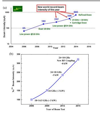
FIG. 22. <sup>209</sup>Bi<sup>31+</sup> (a) and <sup>129</sup>Xe<sup>30+</sup> (b) beam intensity evolution with different technical developments from the year 2006 to 2015.
