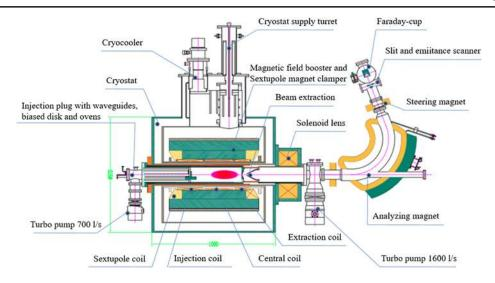
FIG. 2. Layout of the SECRAL ion source and its beam transport line.
