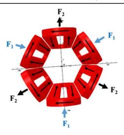
FIG. 6. View of sextupole-coil end in which the adjacent end electric-current flows oppositely. Interaction between the end currents and the axial fields results in strong radially inward force F1 and outward force F2.
