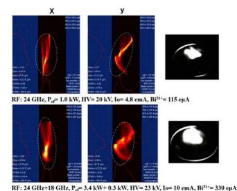
FIG. 25. Beam emittance phase-space patterns and beam images for the beam <sup>209</sup>Bi<sup>31+</sup> at different conditions for SECRAL operating 24 GHz.
