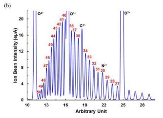
FIG. 12. CSD spectrum with the source optimized for <sup>129</sup>Xe<sup>20+</sup> and <sup>209</sup>Bi<sup>50+</sup>. (a) Xenon CSD spectrum with the source optimized for <sup>129</sup>Xe<sup>20+</sup> at 2.9 kW of 18 GHz microwave power and 25 kV extraction voltage. (b) Bismuth CSD spectrum with the source optimized for <sup>209</sup>Bi<sup>50+</sup> at 2.6 kW of 18 GHz microwave power and 25 kV extraction voltage.
