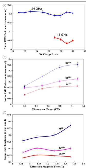
FIG. 23. SECRAL beam emittance study. (a) Xenon beam emittance measured at low microwave power of 24 and 18 GHz. (b) Dependences of normalized rms emittance on 18 GHz microwave power measured at SECRAL. (c) Dependences of normalized rms emittance on the extraction peak field at 18 GHz SECRAL.
