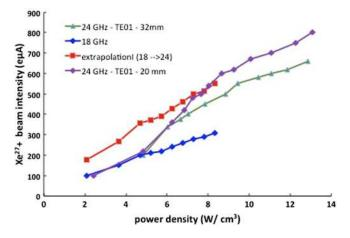
FIG. 19. Dependences of the best beam intensities of  $^{129}$ Xe $^{27+}$  on the total incident microwave power density at 24 + 18 GHz and 18 + 14.5 GHz.
