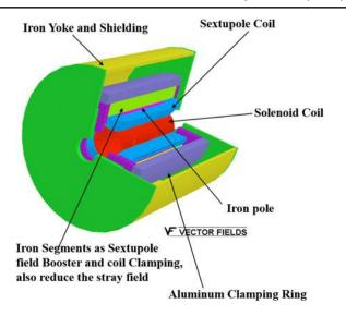
FIG. 7. SECRAL magnet structure and superconducting coil configuration.
