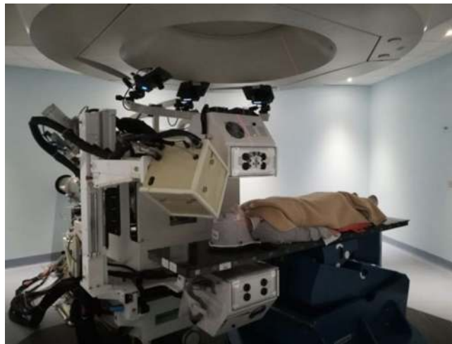
Figure 1. View of the INSIDE cart with the DP (beige box) and the PET detectors (white boxes above and below the patient bed) installed in the CNAO treatment room n.1, which has a fixed horizontal beam line. The image shows a view of the first patient treated with ^{12}\text{C} ions that has been monitored by means of the DP.
