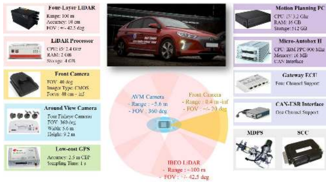
FIGURE 11. Configuration of the test vehicle for implementation of the proposed algorithm.
