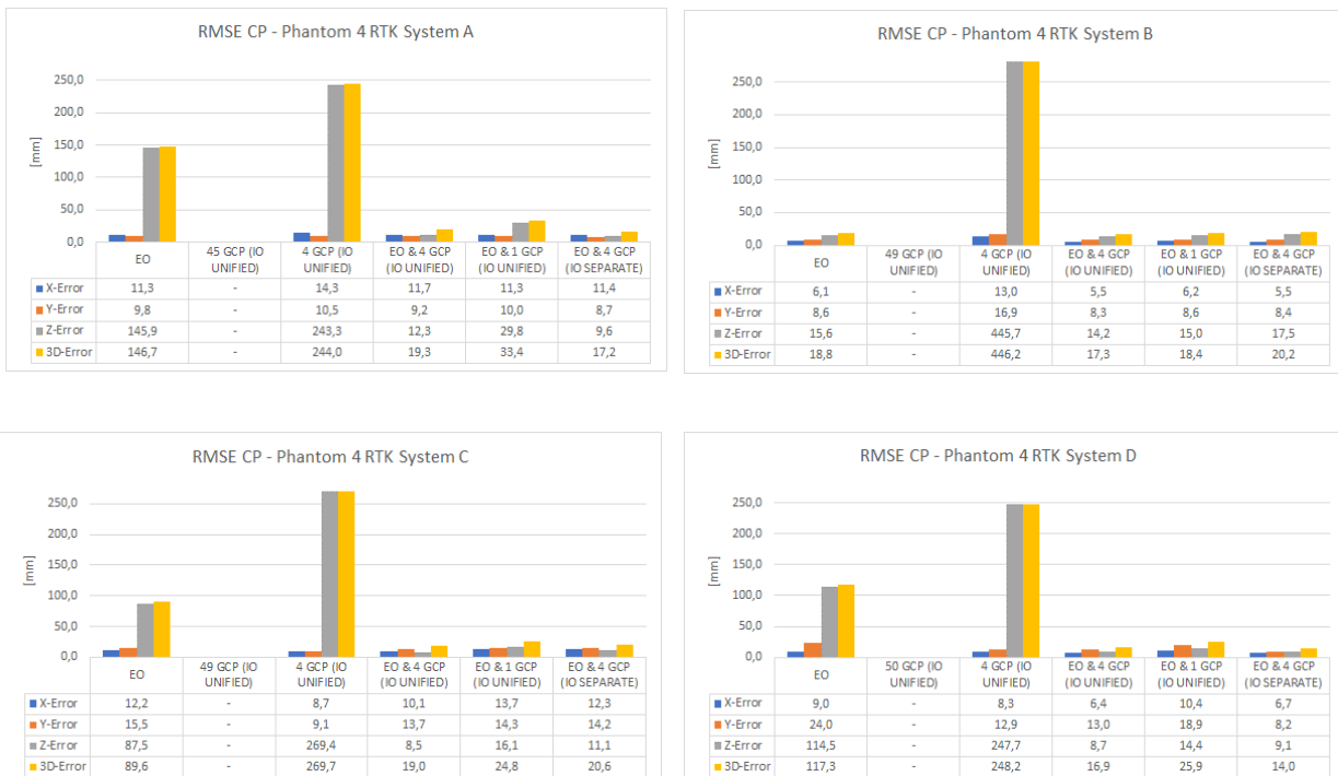
Figure 5. RMSE values at the check points (CP) as a function of the orientation type (direct: EO – indirect: GCP – integrated: EO+GCP) (systems A - D)
