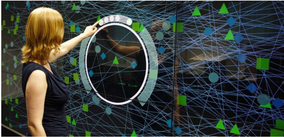
Fig. 9: A graph visualization using the BodyLenses system. The lens provides a personal embodied territory. The user can configure her lens with a touch menu.
