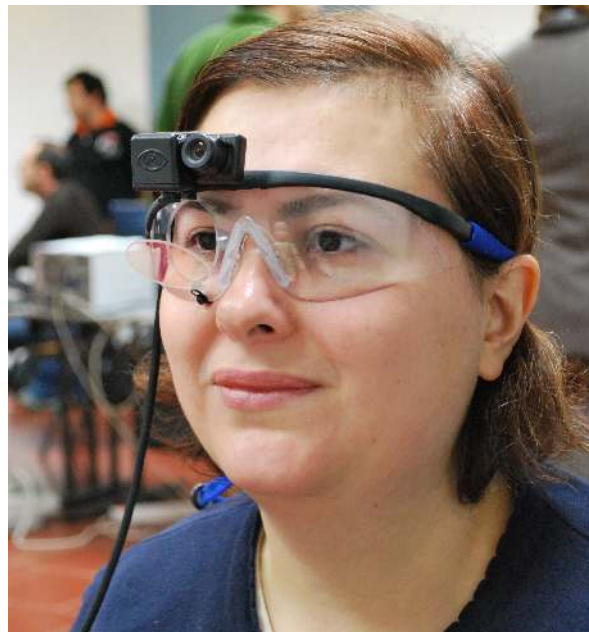
Figure 3. The human interaction partner’s visual attention toward the robot is measured using a gaze tracking system.
