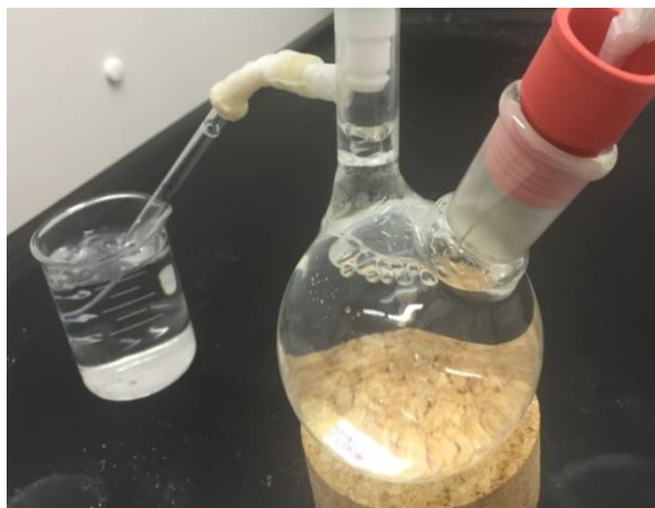
Figure S4. Photograph of the setup used for probing the stability of black phosphorus in DI water with gas ( N_2 or O_2 ) bubbling. Black phosphorus flakes on SiO_2/Si substrate was held in the glass container, in which DI water could either be depleted or enriched in dissolved O_2 .
