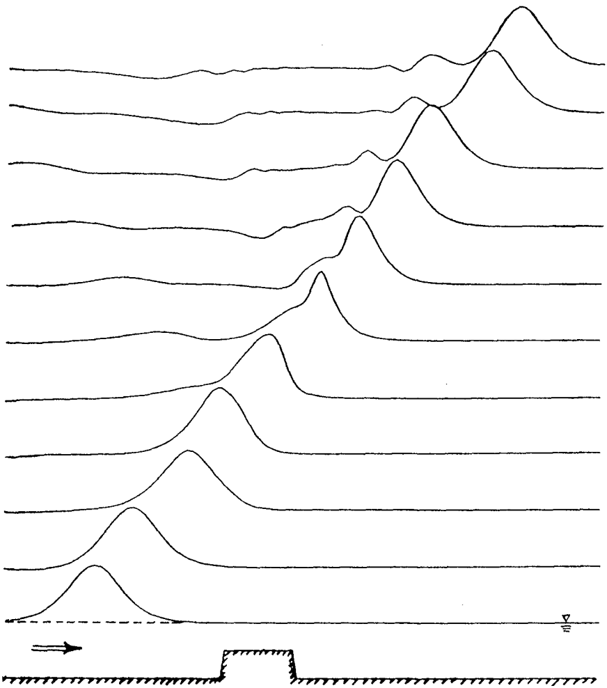
Figure 2: Transformation of solitary wave over submerged breakwater
