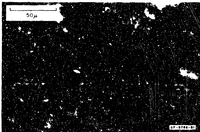
FIG. 56 PHOTOMICROGRAPH OF CERAMIC (AD94) SHOWING FRACTURE
