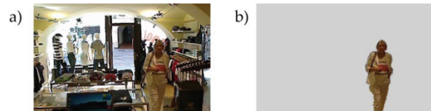
Figure 5. Real-life audience measurement study with the developed system. a) A typical image captured by the digital signage screen unit. b) Image after segmentation described in Section 2.1.
