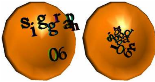
Figure 12: Letters benchmark: Multiple characters interact with a bowl. This model has 3K vertices and 5K triangles. It takes 9.4ms on average for CCD, which is almost 10 times faster than the running time presented in [Sud et al. 2006].
