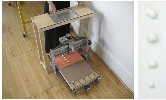
Figure 2. Shaper , a prototype device for interactive fabrication (left) using expanding polyurethane foam (right).
