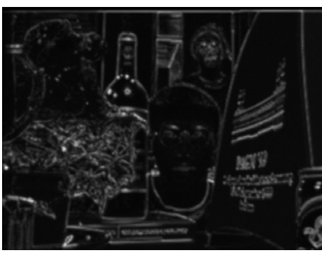
Figure 10: Relative maximum contrast values over all images I . Lighter pixels have high maximum contrast and are likely to be reliable indicators of actual depth.
