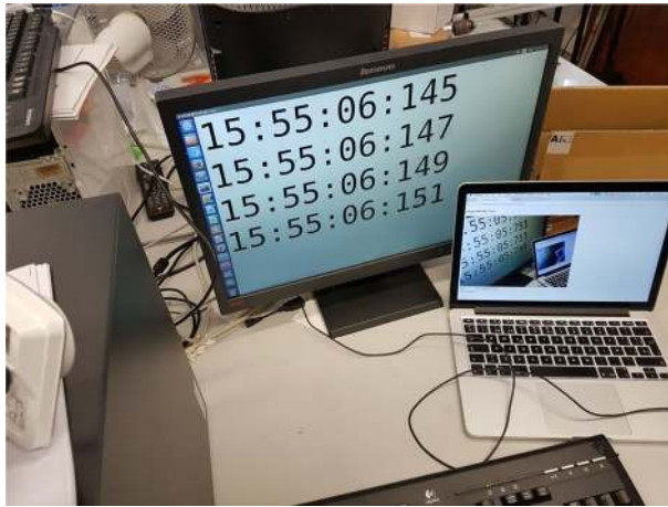
Fig. 5 Picture measuring the capture-render delay
