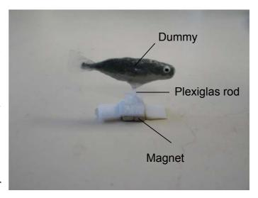
the dummy to live fish and their behaviour can be processed by a computer and behavioural responses of the dummy can be initiated via the robotic arm. This would close the feedback loop and allow interactions with live fish. If small remote-controlled devices are used under the tank to carry electro-magnets instead of a robotic arm, then multiple dummies can be controlled and moved at the same time.
