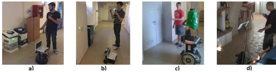
Fig. 1: Robots on which our system has been deployed. a) Turtlebot. b) MARRtino, a mobile base built by our students. c) Mobile base derived from Segway. d) Videre Design platform.
