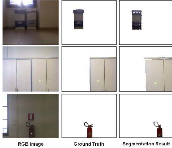
Fig. 3: Three classes of objects have been selected for the quantitative evaluation of the object segmentation module: fire extinguisher, cabinet, and recycle bin. In the first column the images of the objects are reported, while the manually obtained ground truth images for the silhouettes of the objects are shown in the second column. The third column contains the results of the segmentation process.
