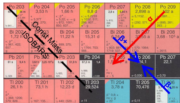
Figure 1 – Nuclide Chart – A section of the Karlsruhe nuclide chart [1]. The decays are shown by the arrows. Elements along the diagonal have the same mass; the sum of neutrons and protons is the same.
