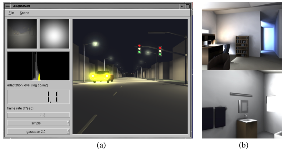
Fig. 2. (a) Our interactive tone mapper for a street scene (70 ktri, 6Hz). The upper left window displays the scene with log colors. The window on the right is used to compute the normalization factor for the weighted average. Below is the histogram of scene luminance. (b) House scene (80 ktri, 6.6Hz). Top: Living room ( 1.4 \log cd/m^2 ). Note the bluish lighting of the adjacent bathroom. Bottom: Bathroom after chromatic adaptation ( 1.8 \log cd/m^2 ).
