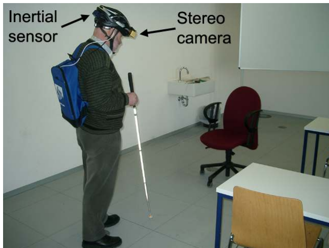
Figure 1: Typical test scenario for the tracking of movable objects. A stereo camera integrated in the front of a bicycle helmet is used for image analysis and distance measurement. The inertial sensor at the back of the helmet provides the current viewing direction. Distance and direction data are used for self-location by comparison with the 3D model, and for detection of differences between reality and model information.
